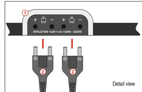
Connect the two plugs (2) on the transformer with the connection sockets (1) on the connector track, **taking care not to reverse the polarity of the plugs and sockets!**
