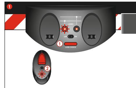
To permit the hand controllers to control the cars, they must once be "bonded" to the connector track. To do this, switch on the racetrack. Both control LEDs on the connector track now light continuously.
